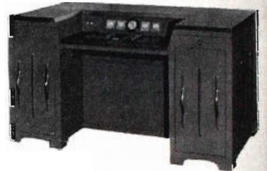
Farnsworth console for control of studio or film television programs, making possible the simultaneous operation of one or more television cameras.
